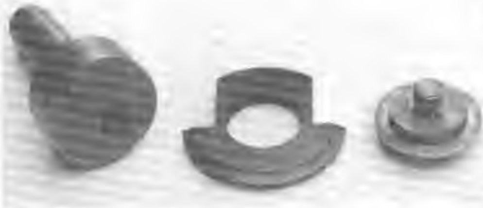
Fig 98 The two flycutters assembled and ready for use.
